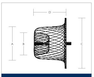
FIGURE I: A: Device diameter at descending aorta. B: Diameter at pulmonary artery. C: Retention skirt diameter. D: Device length. (Figure used with permission from Abbott Cardiovascular, 5050 Nathan Lane, North Plymouth, MN 55442).
