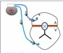
FIGURE 1.1: The normally functioning rateresponsive dual chamber pacemaker (DDD) paces both atria and ventricles in response to activity.
