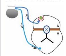
FIGURE 1.2: In sinus tachycardia, the DDD pacemaker senses the atrial activity, tracks it and triggers ventricular pacing.
